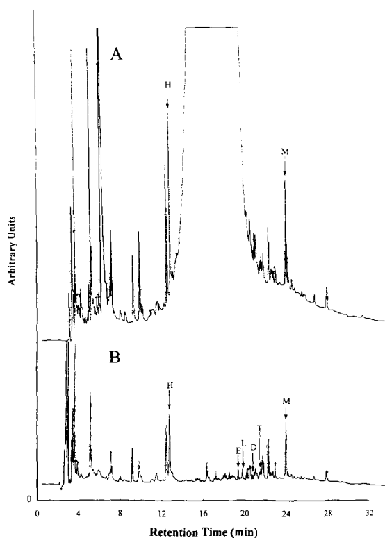
Fig. 2. GC-ECD chromatograms of SFE extractions of a NIST SRM 1941a, a marine sediment: (A) No trapping material in the extraction cell; (B) Using as \text{AgNO}_3 loaded silica as trapping material in the extraction cell. Compounds: H: HCB, E: 4,4'-DDE, L: dieldrin, D: 4,4'-DDD, T: 4,4'-DDT, and M: mirex. See Section 2.3 for extraction conditions.
